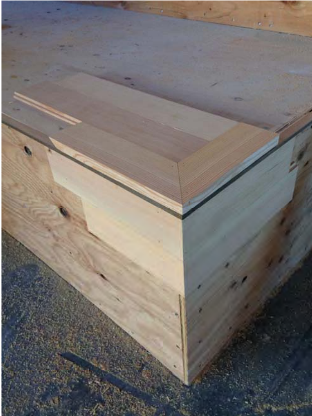
Mock-up of atrium stair finish sample
